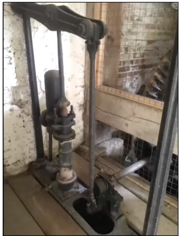
Figure 28. Morland's 'pretty engine' in Euston Mill. The rotating horizontal shaft drives an eccentric wheel causing the vertical rod to rise and fall. The rocker bar transmits the motion to the pump rod. Photo by Steve Temple.
